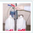
Undo cap on new bottle and carefully place in feed pipe
