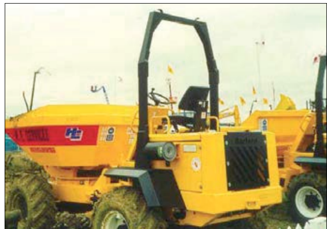
Figure 21 Rollover protective structure (ROPS)
