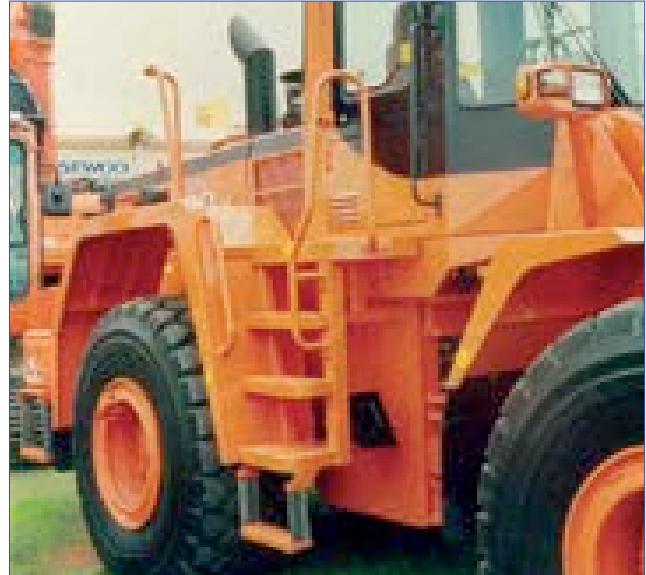
Figure 18 Access to vehicles – steps and handrails
