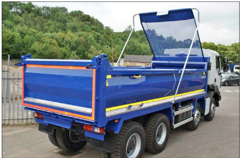
Figure 20 Front-to-rear sheeting system
